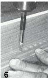
6. Place mylar tape over the score line provided for flange drilling on the beechwood damper tray, and centerpunch each of the markings on the tape. Note: don't confuse the recess for the flange keeper wire with the score line for drilling flange screws! Do this operation in the MIDDLE of the damper tray, leaving plenty of room on either end for trimming and for spring return extensions.
