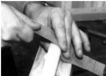
The easiest way to do this is to "gang file" the hammers before they are hung. Place one-third of the hammers at a time into the hammer clamp, and secure this clamp in a vise.
