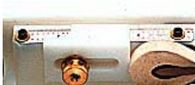
When drilling hammers that are less than 7/16" wide, you may have to loosen the Vice Knob to keep adequate pressure on the hammer.
