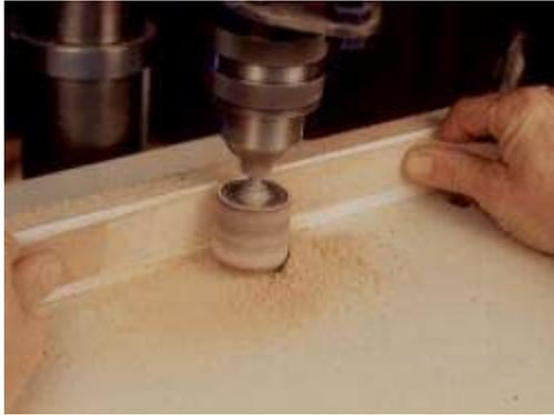
Photo #6 - sanding leather thickness
