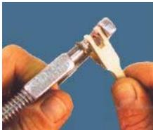
1. Unpin the old part(s), measure and note the original pin size.
