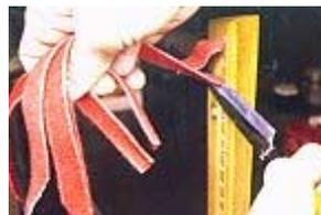
6. Size the bushings by wetting with alcohol and inserting a #7 bridge pin into each. Most damper wires measure .073", and #7 (.086") bridge pins size the bushings to a comfortably free fit. If you prefer a tighter fit, use #6 (.076") bridge pins. Place in a warm spot to dry for several hours. When the bushings are thoroughly dry, they will have uniform, firm holes free of fuzz that will control the damper wires with negligible friction.
