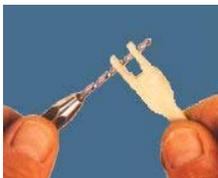
3. Clean out the bushing holes using the proper sized drill in a pin vise. For most parts, this will be a #37 drill (.104"). You want to remove only cloth and glue residue, and not damage the wood. Best results are had by first turning the drill counter clockwise until it is through both flange ears, then forward a turn or two. This maintains the original alignment of the two holes.
