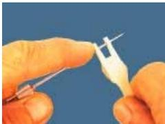
8. Test the fit of the pin in the bushing. Usually it will feel quite tight. Avoid reaming if possible; you will get a denser, more solid bushing if you compress the cloth with a smooth tapered burnisher since coarse reamers tend to loosen up the cloth. Rotating the burnisher slightly, slip it into one side of the bushed part. Note the distance with your finger on the burnisher, then insert into the other side the same distance.
